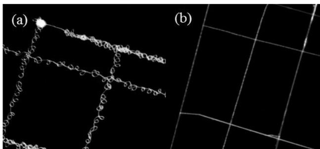
**Figure 3.** Transition from an unstable nanofiber jet at 600V (a) to a stable controlled jet at 300V (b) allows easy patterning
