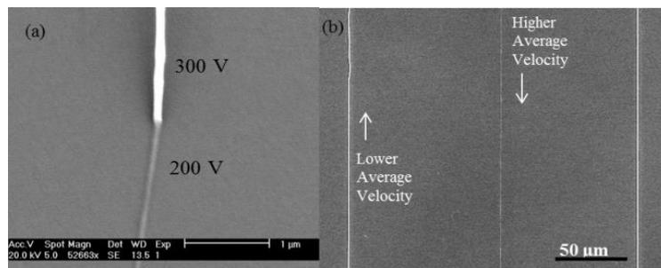
**Figure 4.** Applied voltage and stage speed are used to control nanofiber thickness in the EMS technology
