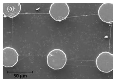
Figure 2. Direct wiring of 3D micropost structures with EMS.
